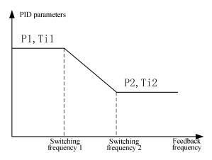
Fig. 7-21 Schematic Diagram of PI Parameters
