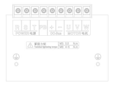
d) Schematic Diagram of Terminals (EM730-030-3/3B~EM730-037-3/3B)
