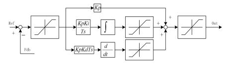
Fig. 7-27 Block Diagram of Process PID
