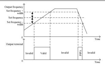
Fig. 7-36 Schematic Diagram of FAR Detection
