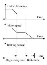
Fig. 7-17 DC Braking Process for Start
