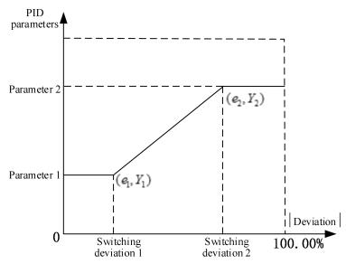
Fig. 9-28 Schematic Diagram of Automatic Switching of PID Parameters based on Deviation (F19.11=2)
