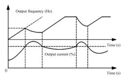
Fig. 7-25 Current Limit Process
