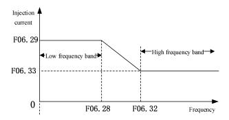
Fig. 7-22 Schematic Diagram of High Frequency Injection
