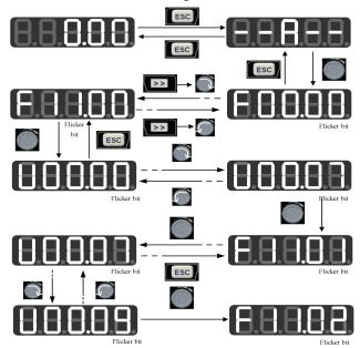
Fig. 4-4 Example of User-defined Mode Setting
