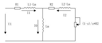
Fig. 7-11 Steady-state Equivalent Model of Asynchronous Motor
