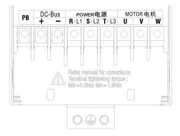
b) Schematic Diagram of Terminals (EM730-2R2-3B~EM730-4R0-3B)
