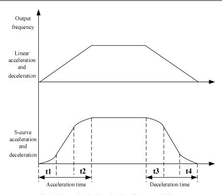
Fig. 7-16 Acceleration/Deceleration Time Control Diagram
