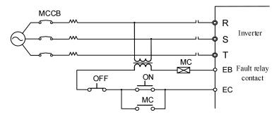
Fig.3-4 Connection of Input Circuit Breaker
