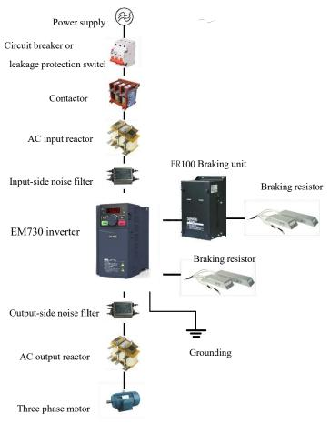
Fig.3-1 Connection of Inverter and Peripheral Devices
