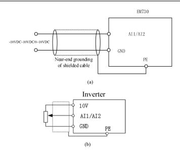
Fig.3-12 AI1/AI2 Terminal Wiring Diagram
