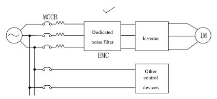
Fig.3-5 Correct Installation of Noise Filter
