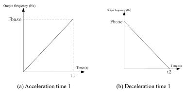
Fig. 7-9 Acceleration and Deceleration Time
