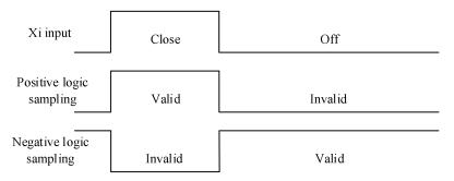
$Fig.\ 7\text{--}12\ Schematic\ Diagram\ of\ Positive/Negative\ Logic\ Sampling\ of\ Terminal$
