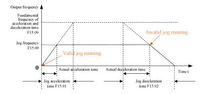
Fig. 7-32 Schematic Diagram of Jog Running
