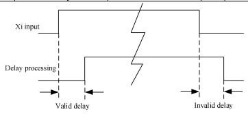
Fig. 7-14 Schematic Diagram of Terminal Delay Sampling
