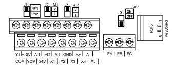
Fig.3-11 Layout of Control Circuit Terminals 1
