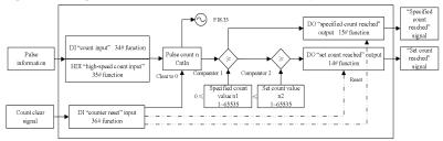
Fig. 7-42 Block Diagram of Counting Function
