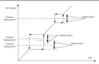
Fig. 7-35 Schematic Diagram of Frequency Hopping
